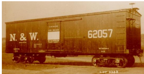
Built by ACF's Huntington Shops in 1904, these double sheathed N&W boxcars were among the first in the country built with steel body framework. ACF builder's photo, St. Louis Mercantile Library collection.
