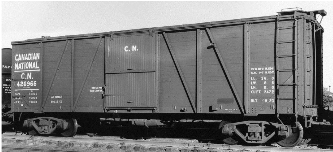
CN car with six foot door. The cars was built in 1923, and by the time of this 1957 photo had been modernized with an outside metal roof, cast steel trucks, and AB brakes.
